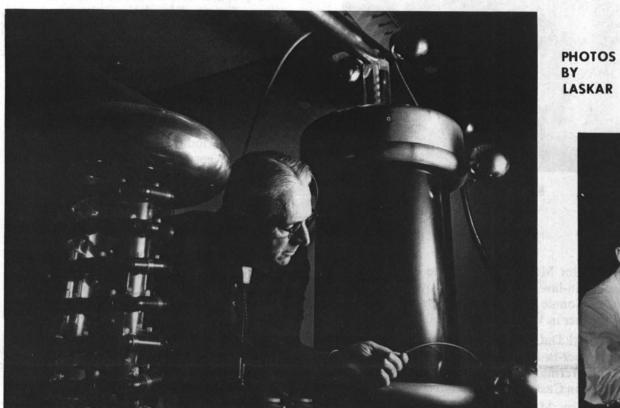
BOB McCALLUM works on equipment in the high voltage laboratory before calibrating high voltage divider instruments.
